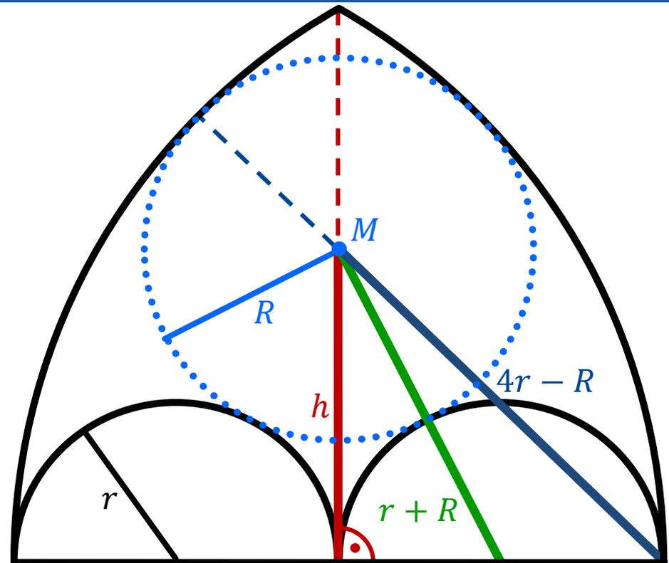
$$\left. \begin{array}{l} (1) \quad h^2 = (r + R)^2 - r^2 \\ (2) \quad (4r - R)^2 = h^2 + (2r)^2 \end{array} \right\} \begin{array}{l} \text{Einsetzen von} \\ (1) \text{ in } (2) \text{ liefert:} \end{array}$$
